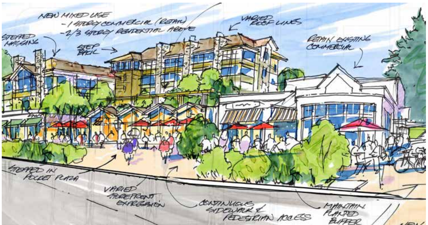
Building heights are generally limited to three storeys and may be up to four storeys with specific step-backs of the building and the provision of public amenity space.
